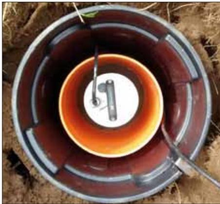
3 (Above) Seismometer installed in the ground at Sherbrooke Nova Scotia, part of the Maritimes QM-III deployment. (Amy Gilligan)
